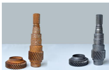
Gear rust removal
